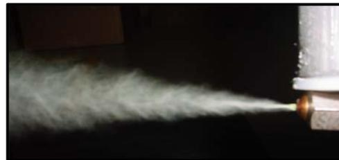
Figure 9: Aerosol sealant product being tested to reduce air infiltration and improve building efficiency.
